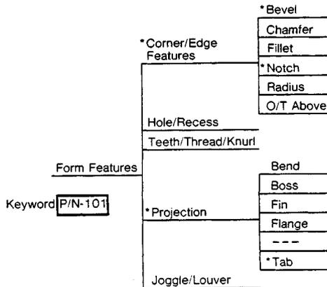
**Fig. 31.3** N-tree concept applied to form features.
