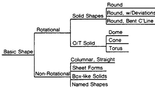
Fig. 31.2 E-tree concept applied to basic shape classification.
