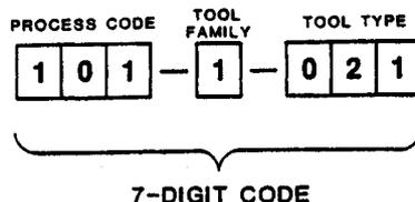
Fig. 31.29 Fabrication tool code format.
