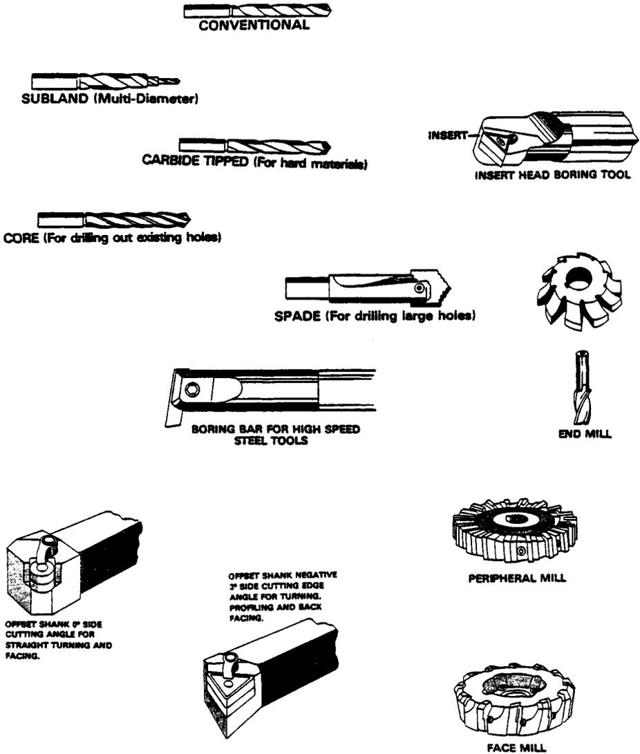
Fig. 31.27 Standard tooling.
