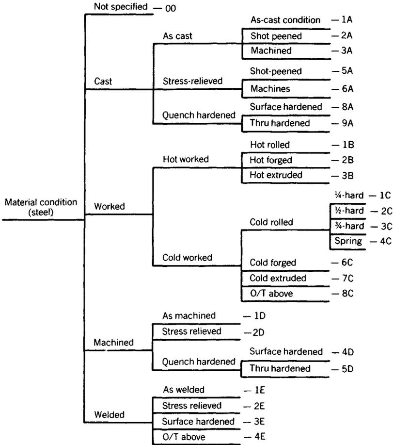
Fig. 31.13 Material condition for steel family "A1."
