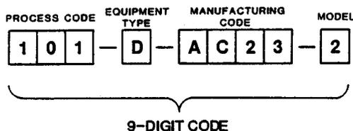
Fig. 31.24 Fabrication equipment code.
